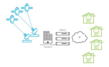
By offering open standards DVB-Common Interface multi-service descrambling capability in conjunction with DVB-S/S2 and MPEG-2 and 4 Multi-Format capability the RX8315 ensures that all services can be reliably ingested into the DTH delivery platform.
